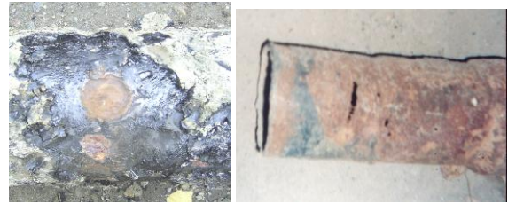
Fig. 11. Deterioration of underground metallic pipelines caused by stray currents
