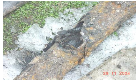
Fig. 11. Deterioration of underground metallic pipelines caused by stray currents
