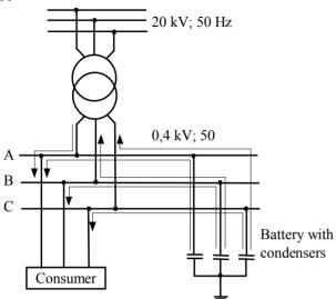
Fig. 1 – The circulation of the reactive power on the three phases of the analyzed consumer.
