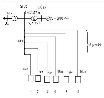
Fig 4. The distribution network with six lines and one task per each line.
