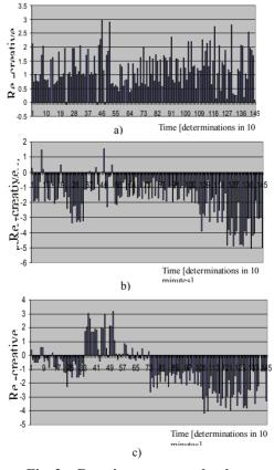
Fig. 2 – Reactive power on the three phases of transformer (low voltage part):
