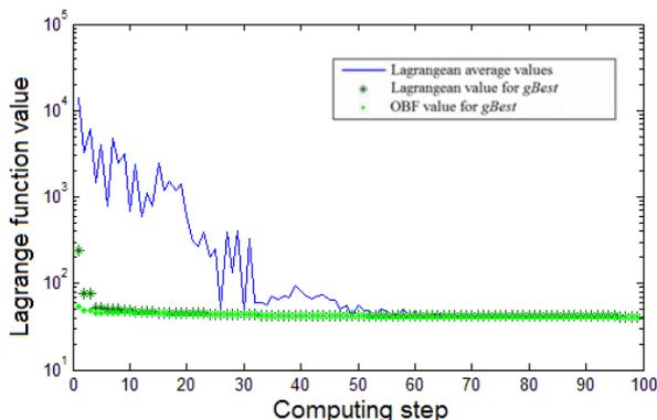
**Fig. 5. PSO algorithm evolution for OPF computing**
