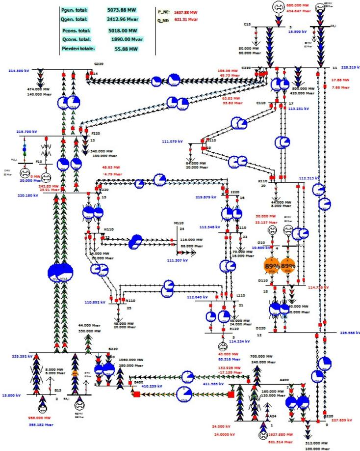
Fig. 4. Maximum expansion solution one-line diagram
