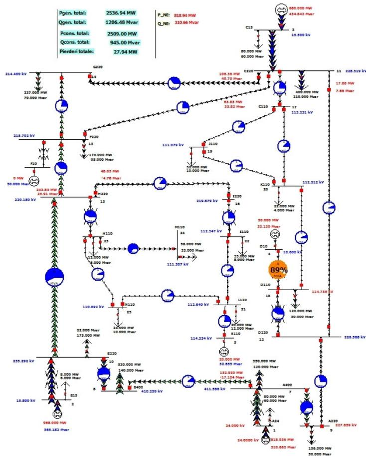
Fig. 3. Test 25 buses test power system – one line diagram
