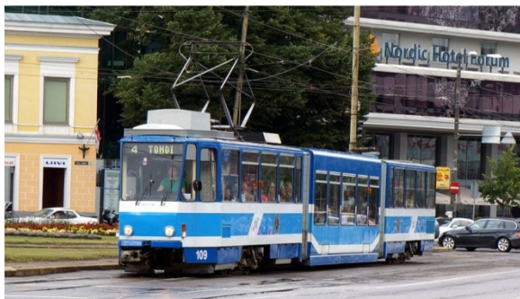
Foto 2. TATRA KT4 adapted to Low-Floor in TALLIN-Estonia
