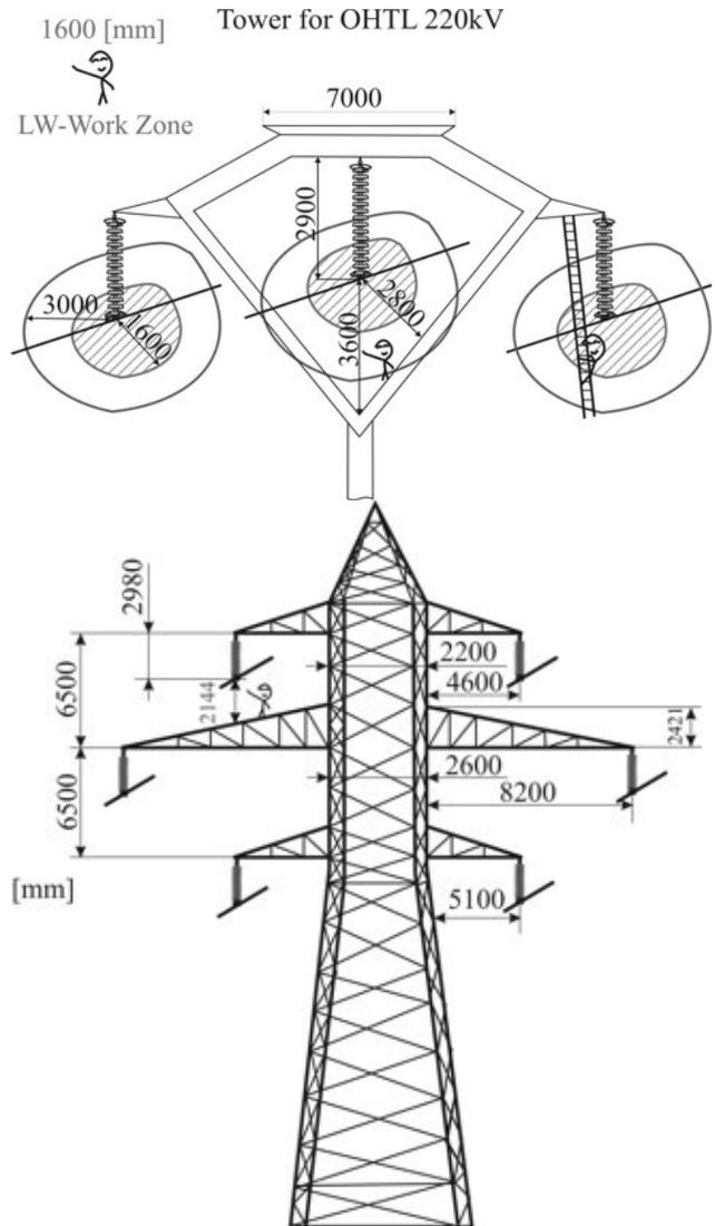
**Fig.3. Clearance distances for works at 220kV OHTL**
