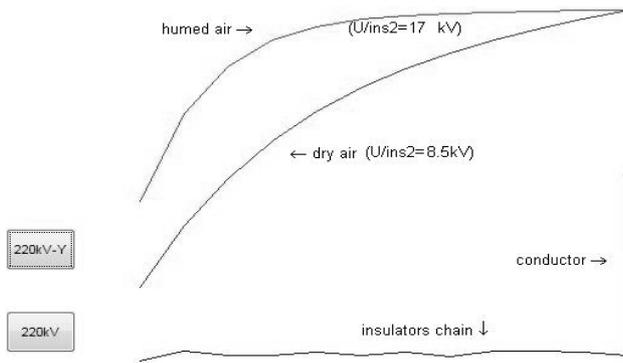
**Fig.4. Voltage distribution in a chain of glass insulating type to a 220kV tower, "Y" type**
