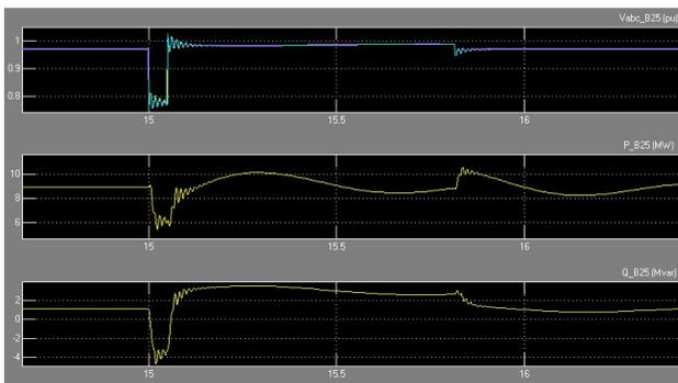
**Fig.8. Three-phase fault on line that supplies the consumer 3**
