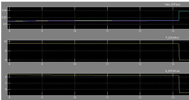
**Fig.7. Grid operation with compensator STATCOM disconnected**
