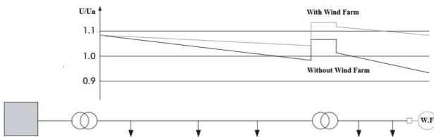
**Fig.3. The influence of wind groups on the profile voltage in an electrical distribution grid**
