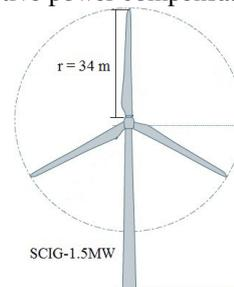
**Fig.4. Wind turbine - 1.5 MW equipped with squirrel cage induction generator**
