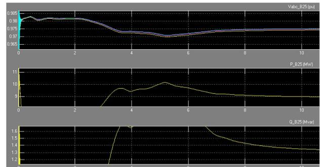
Fig.5. Grid operation with compensator STATCOM connected
