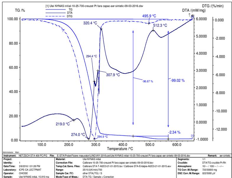
Fig. 4. TG – DTA and DTG thermograms registered for Nynas sample before cycling
