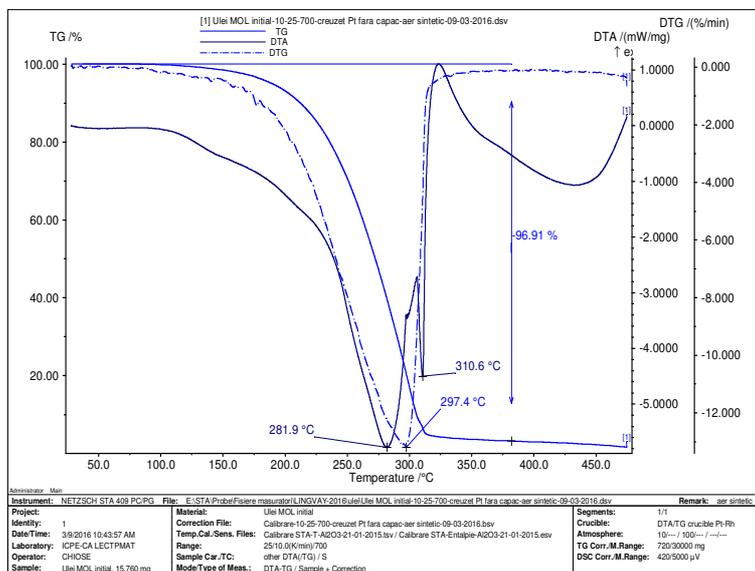
Fig. 6. TG – DTA and DTG thermograms registered for MOL TO 30 oil sample before thermal cycling
