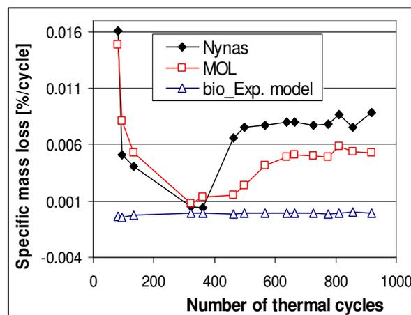
Fig. 3. The variation of specific mass losses over the thermal cycling
