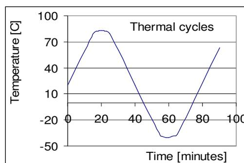
Fig. 1. Thermal treatment profile of applied cycles (thermo cycles)
