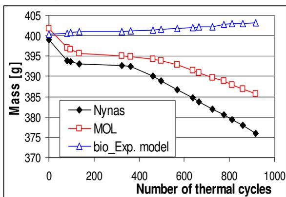
Fig. 2. Variation of samples' mass over the thermal cycling
