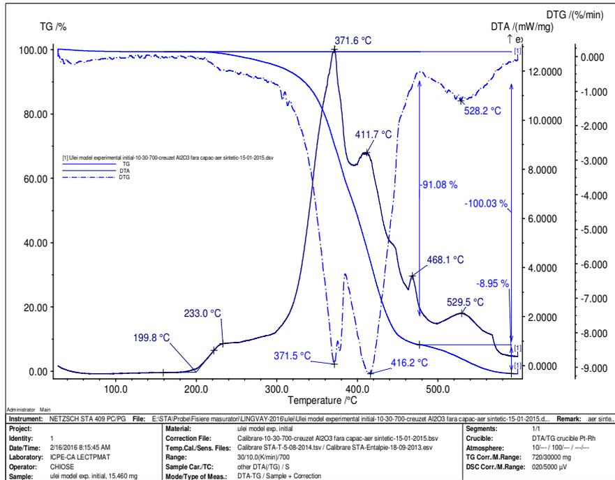
Fig. 10. TG – DTA and DTG thermograms for the sample of experimental model of oil before thermal cycling
