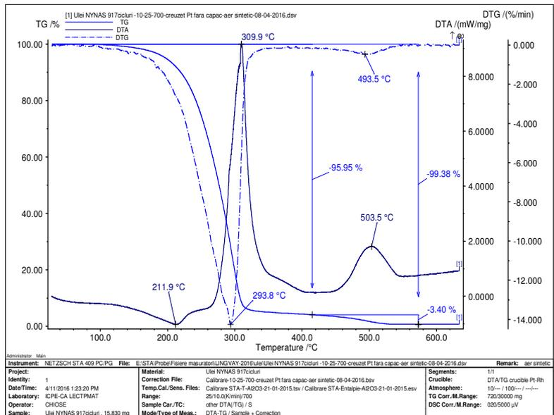
Fig. 5. TG – DTA and DTG thermograms registered for Nynas sample after 917 cycles (Fig. 1)
