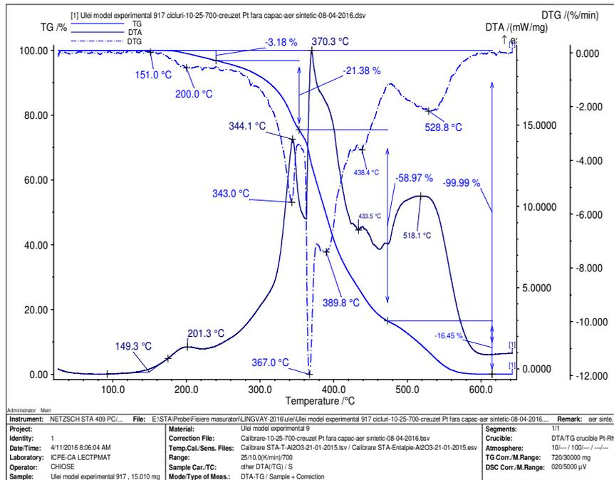
Fig. 11. TG – DTA and DTG thermograms for the sample of experimental model of oil after applying 917 thermal cycles (Fig. 1)
