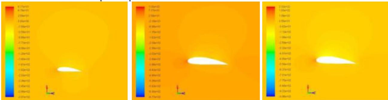
**Fig. 12. The pressure coefficients field for NACA 4418 profile for specific speeds: a.  $\lambda=5.02$ ; b.  $\lambda=2.51$ ; c.  $\lambda=1.67$ .**
