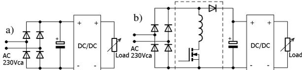
Fig. 6. AC/DC rectifier in PC power supplies a) with no power factor corrector (PFC), b) with PFC block
