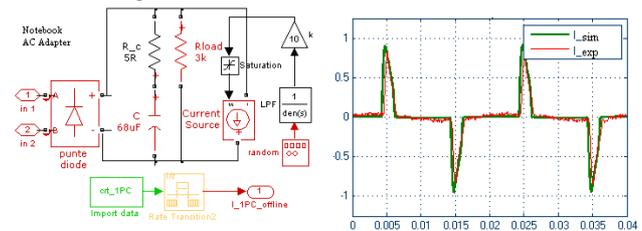
Fig. 8. a) Simulation model for notebook AC adapter, b) Comparison between experimentally measured current and the simulated one
