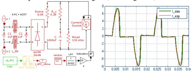
**Fig. 10. a) Simulation model for a group of 4 PCs, b) Comparison between experimentally measured current and the simulated one**
