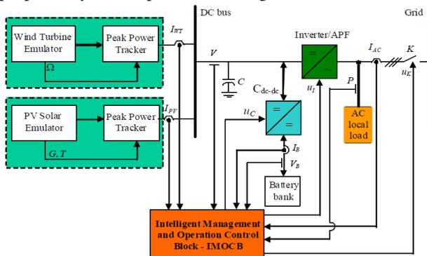
**Fig. 1. Structure of the proposed distributed power system**
