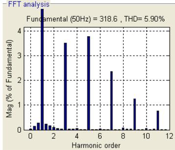
Fig. 5. Harmonics content of the grid voltage
