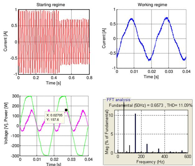
Fig. 15. Experimental signals for a 40W classical fluorescent lamp
