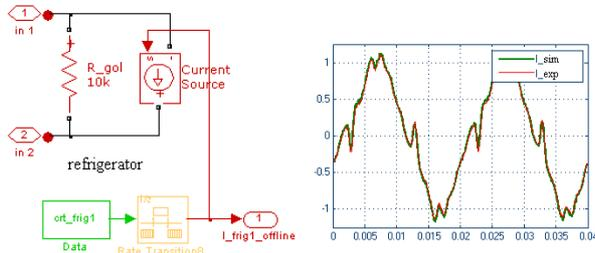
**Fig.18. Simulation model and comparison with experimental signals for a refrigerator**
