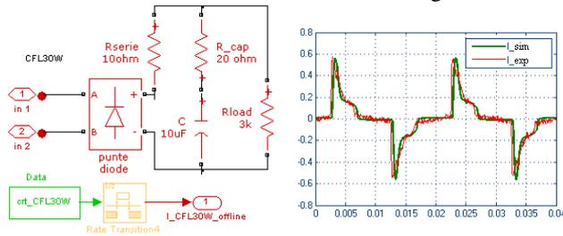
Fig. 14. Simulation model and comparison between simulation and real current waveform
