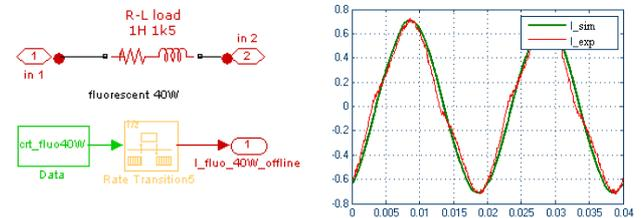
Fig.16. Schematic and comparison with experiment for the classical fluorescent lamp
