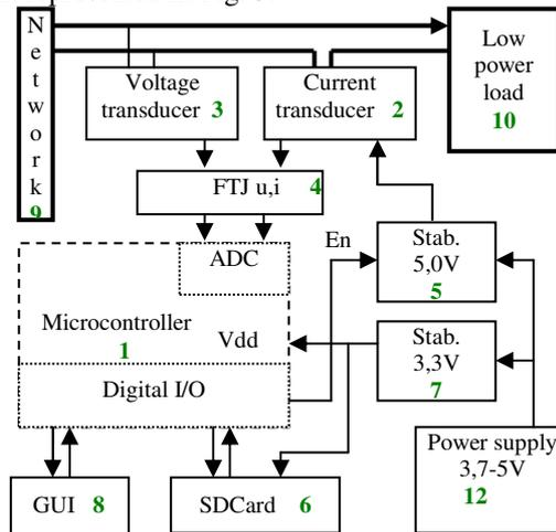
Fig. 2. Structure of the DATALOG circuit
