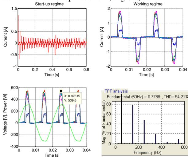
**Fig. 9. Signals of interest for a desktop PC power supply**
