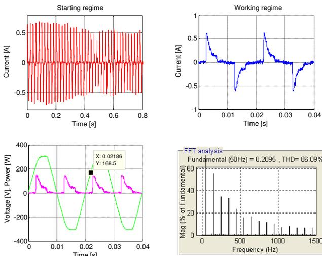
Fig. 13. Experimental signals for 26W CFL
