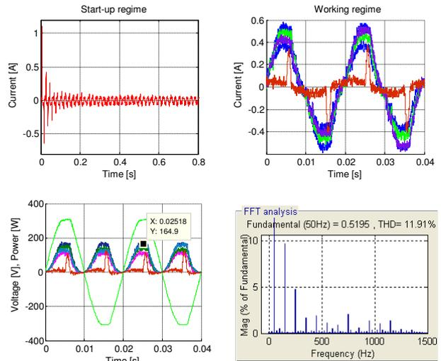
**Fig. 11. Signals of interest for a PC power supply with power factor correction circuit**
