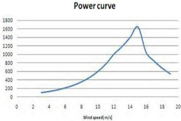
**Fig. 3 The wind power curve for small power wind turbine.**
