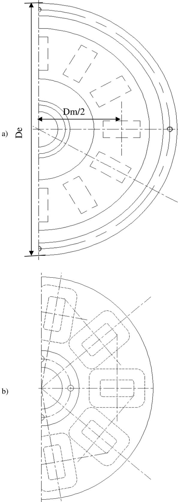
**Fig.5 a) The placement of permanent magnets on the rotor; b) the placement of coils on the stator,  $D_e$  is the outer diameter of the rotor, and  $D_m$  is the average diameter for placing the permanent magnets and the stator coils.**
