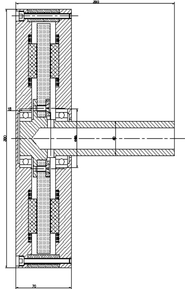
Fig. 8 The final dimensions of the designed prototype of permanent magnet axial wind generator.
