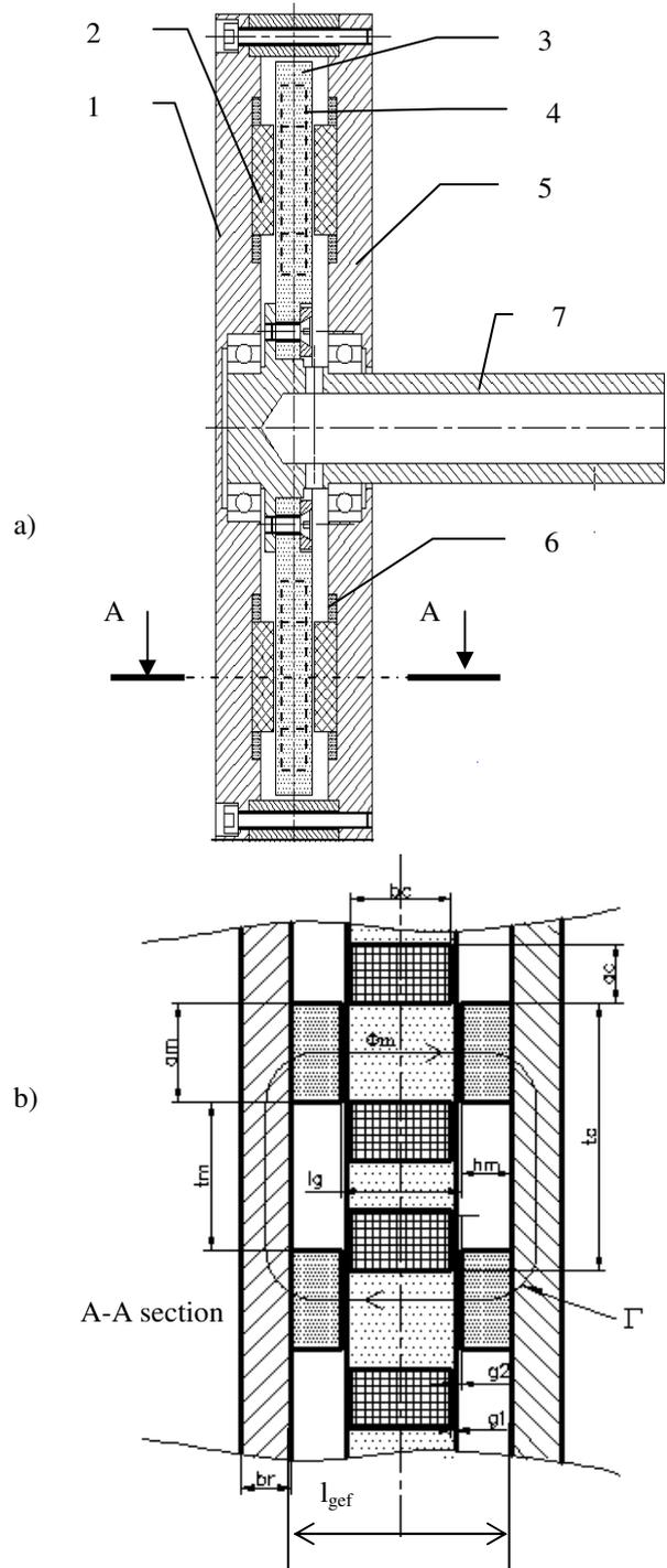
**Fig. 4: a) The axial flux permanent magnets wind generator with iron free stator: 1 - rotor 1; 2 – permanent magnets, 3 – stator; 4 – coils; 5 – rotor 2; 6 – epoxy resin; 7 – ax; b) the cross-section through the rotor.**
