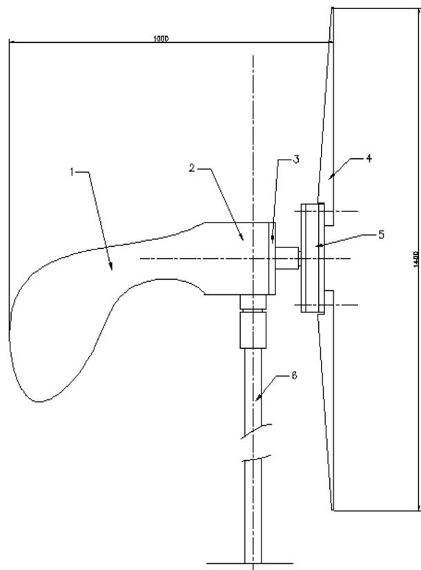
Fig. 2: The wind turbine for residential application: 1 – orientation vane; 2 – nacelle; 3 – support; 4 – blade; 5 – wind generator; 6 – mast.
