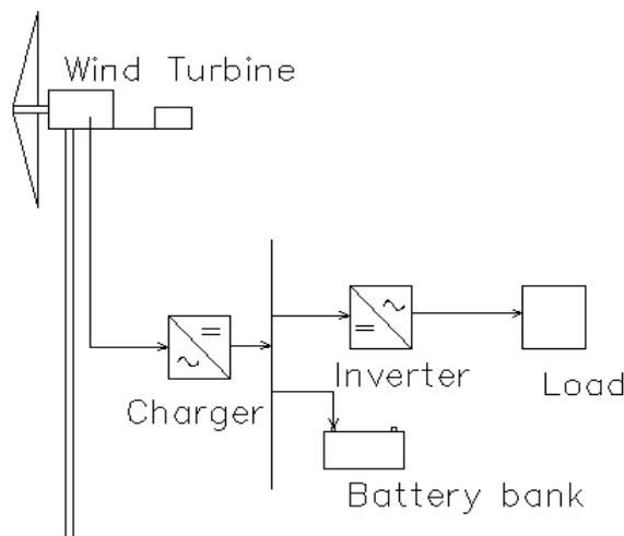
Fig. 1: The structure of an off grid wind turbine.
