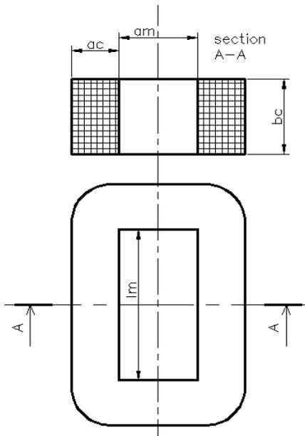
Fig. 6: The coil shape.
