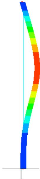
Fig. 3 - The shape deformation for mode 2
