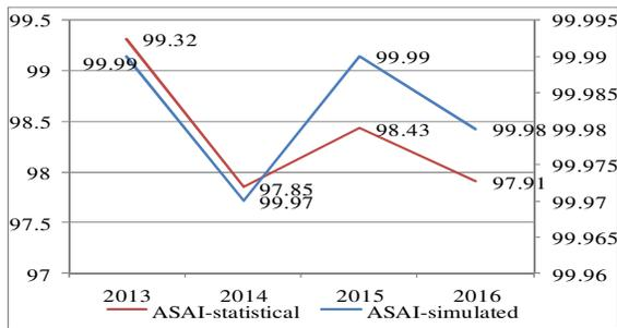
**Fig.10. Availability index for the power transformers in the power transmission of Kosovo (2013-2016)**
