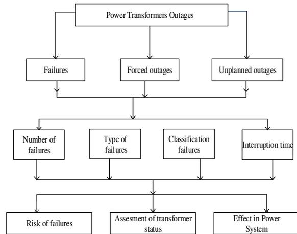
**Fig.3. Factors for security and reliability assessment and transformer operation**
