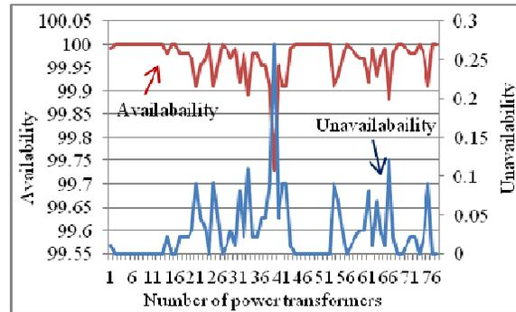
**Fig.1. Availability and unavailability of power transformers in the power transmission system of Kosovo**
