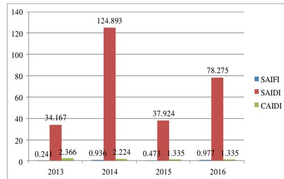
Fig.8. Monitoring of power transformer reliability indicators for peak load 1090 MW based on outages with single mode failures
