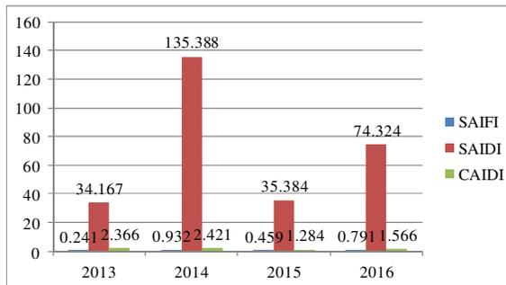
Fig.9. Monitoring of power transformer reliability indicators for peak load 650 MW based on outages with single mode failures
