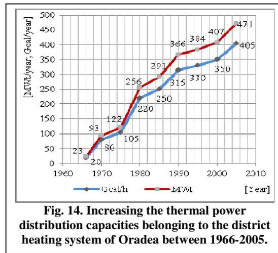
**Fig. 14. Increasing the thermal power distribution capacities belonging to the district heating system of Oradea between 1966-2005.**
