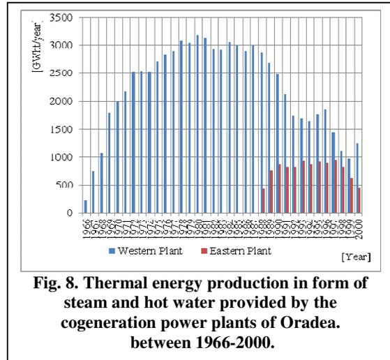
**Fig. 8. Thermal energy production in form of steam and hot water provided by the cogeneration power plants of Oradea. between 1966-2000.**
