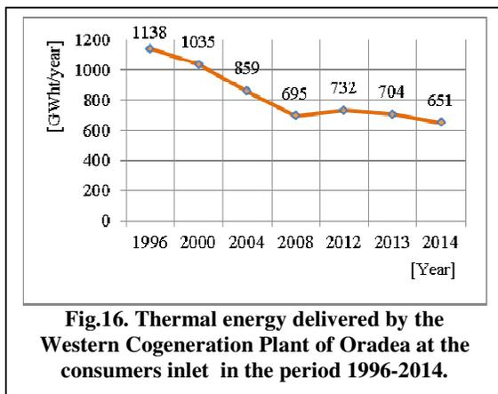
Analyzing the values of the thermal energy delivered from the Western Cogeneration Plant between 1996-2014, measured at the inlet of the consumers equipments, there is a continuous decrease of the supplied heat during 1996-2008, from 1,130 GWh/year to 690 GWh/year, which then will stabilize by 2014 around the values of (680-700) GWh / year, as results from the figure 16, [5].
