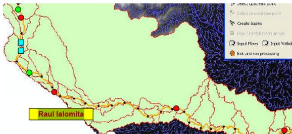
**Fig. 3. The necessary data of the Ialomita river: red-measured, blue-captured, green-returned flow rate**
