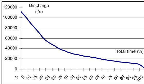
**Fig. 6. The Flow duration curve**
