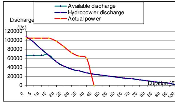
**Fig. 8. Flow and Power duration curves**
