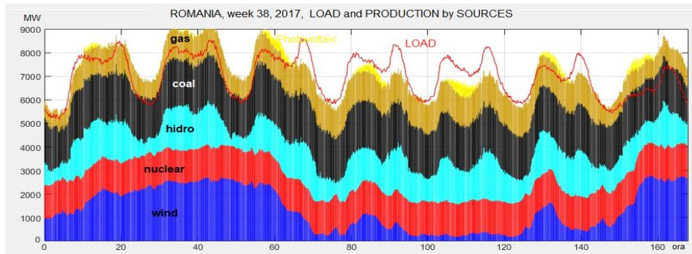
Figure 8. Electricity production in Romania, in week 38, 2017 by sources towards consumption
