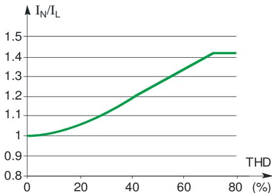
Fig. 6. Charging of the null conductor for unbalanced loads
