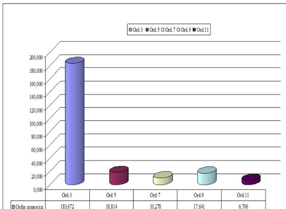
Fig. 7. Spectrum of harmonics through the null conductor in PTab 2 - 20 / 0.4 kV
