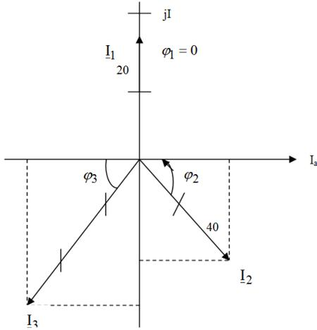
Fig. 9. Phasor diagram of the unbalanced network
