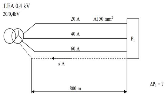
Fig. 8 Unbalanced current network
