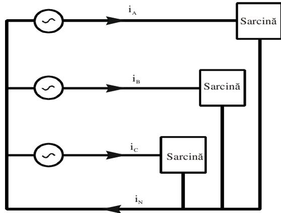
**Fig. 3. Balanced single-phase loads**
