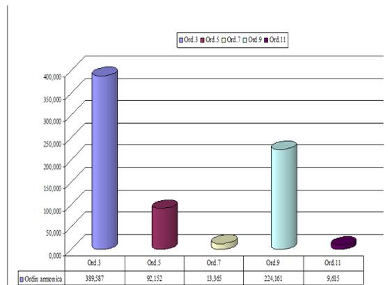
Fig. 2. Spectrum of harmonics through the null conductor in PTab 3 - 20 / 0.4 kV
