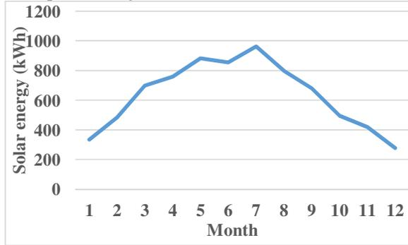
**Fig.6. Supplied solar energy for space heating and DHW**
