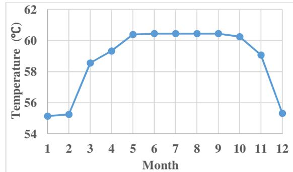
**Fig.5. DHW storage maximum temperature of the proposed system**
