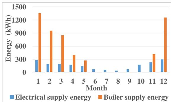
**Fig.7. Supplied electrical and boiler energy for the proposed system**
