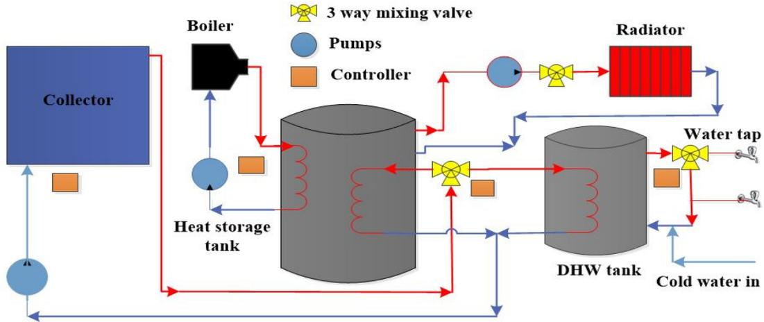
**Fig. 1. Space and domestic hot water system for residential application**
