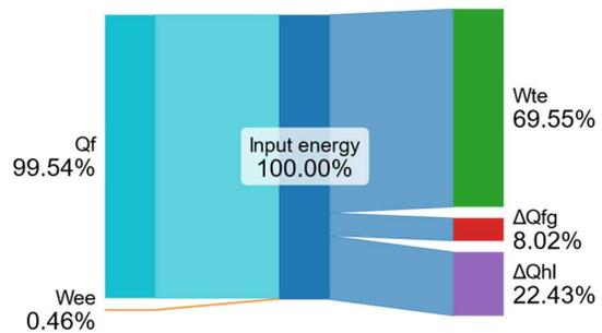
**Fig. 4. Sankey diagram for the EB performed for Case 2**
