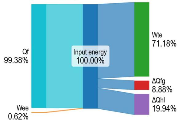
**Fig. 3. Sankey diagram for the EB performed for Case 1**
