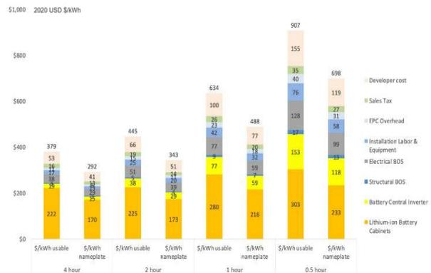
Fig. 21. U.S. utility-scale Li-ion battery stand-alone storage costs for durations of 0.5–4.0 hours (60 MWDC), Q1 2021 [39]
