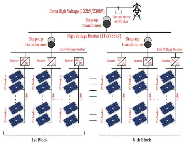
Fig. 2. Block diagram of a utility-scale solar power plant
