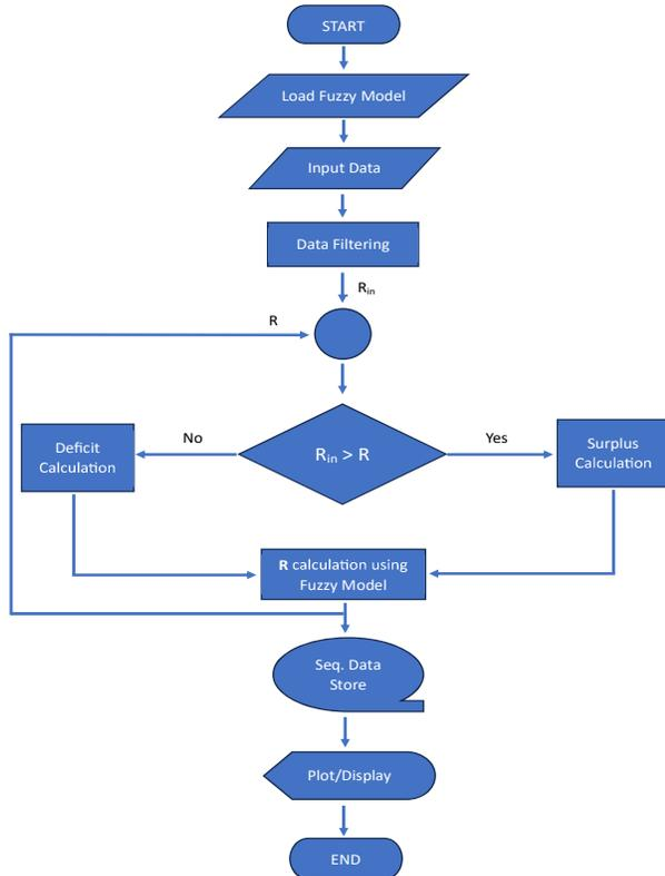
Fig. 6. Block diagram of the data analysis process
